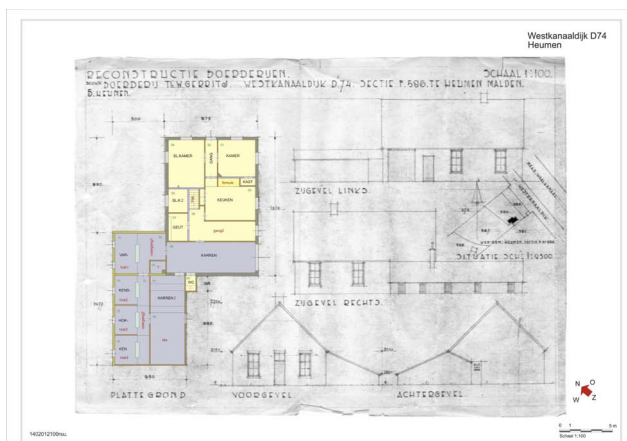
Illustration 2. Architectural drawing of Westkanaaldijk with vectorized plan and labelled spaces.
