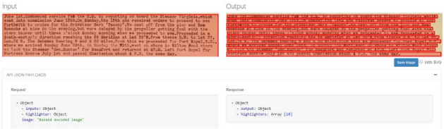
Figure 6 Results of a text line segmentation method. User input (left) is shown together with the computed results (right). Below the images is the JSON information a programmer would receive when calling the methods on DIVAServices directly.
